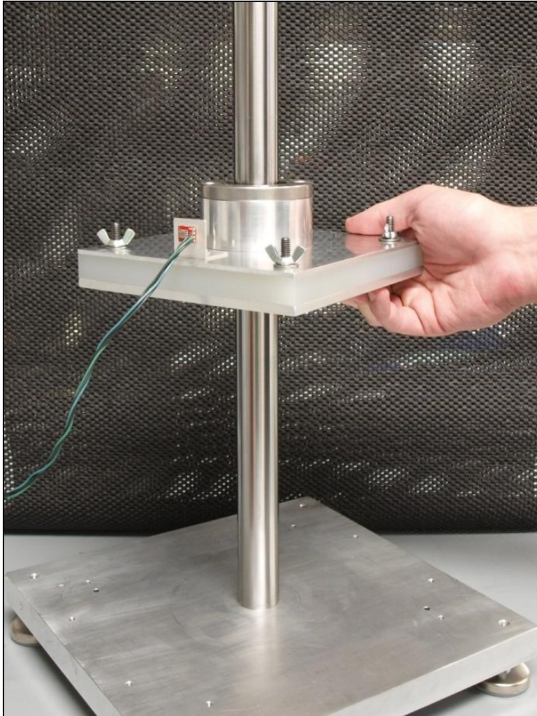
Figure 1: Assembled shuttle rose manually from the impact base and guided by a fixated rod. Mounted accelerometer is wired to a BUS-powered DAQ and PC not shown. The orientation of the accelerometer's single strain gage rosette is the same as the fixated rod: normal to the impact base. Photograph was taken by Zachery Heller.
